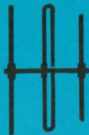
109 3-Element array with folded dipole
