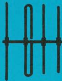
113 4-Element array with folded dipole
