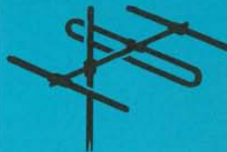
203 3-Element array with folded dipole
