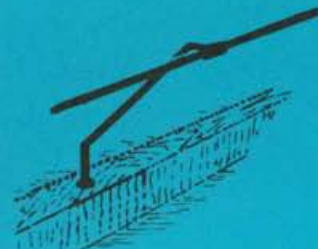
205 L Dipole for loft mounting
