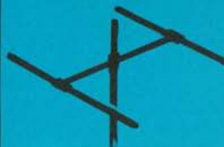
202 Dipole with single reflector
