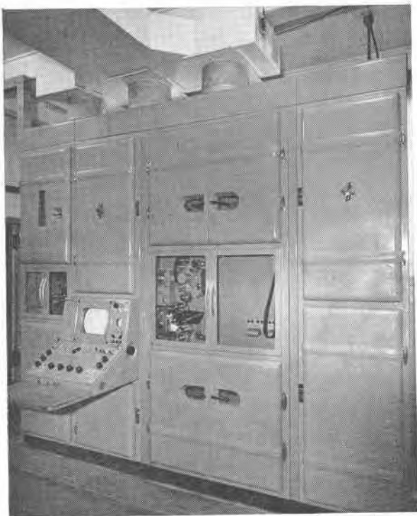
Two examples of film scanning equipment using the flying-spot principle. In the equipment shown movement of the film is continuous. Other types
