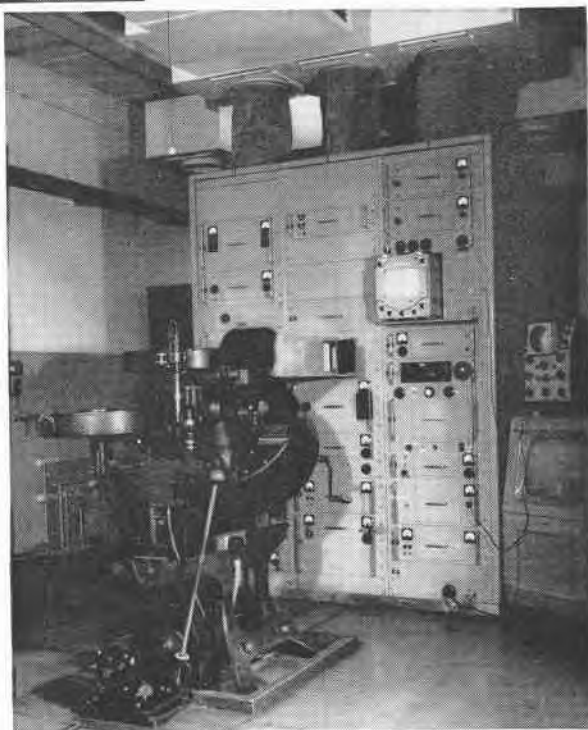
Two examples of film scanning equipment using the flying-spot principle. In the equipment shown movement of the film is continuous. Other types
