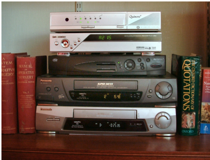
Fig 5. This B-Tech Quintro+ automatic scart switch (top) presides over the customer's motley collection of satellite receivers and VCRs. The Quintro has five RGB/composite inputs. These can be selected automatically or manually for routing to the TV set. At the same time the device can route signals between input devices for recording. Automatic scart switchers provide a good solution when the TV set hasn't enough A/V inputs.
