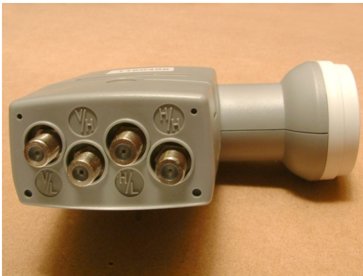
Fig 11. A quattro LNB. The four outputs are fixed: vertical low band, vertical high band, horizontal low band, and horizontal high band.
