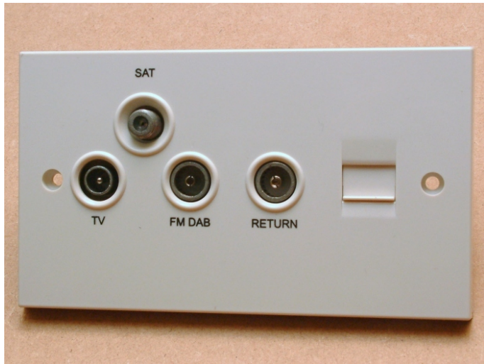
Fig 9. Typical of the various makes of 'master' wallplate, this Labgear PSW242T includes a triplexed satellite/UHF/VHF outlet, a socket for the return feed to other rooms, and a phone socket.
