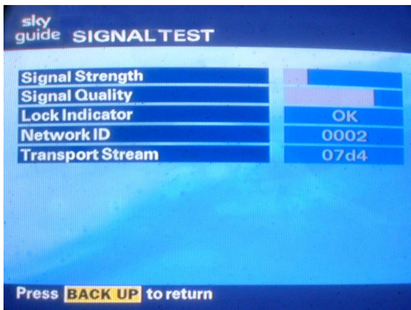
Fig 18. The Signal Test display of a Sky receiver. Some residents will query the low signal strength indication, but it has no real significance.
