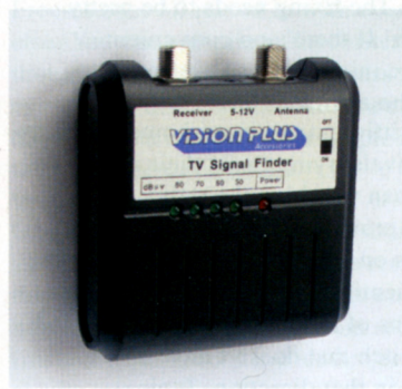
The Vision Plus TV signal finder from Status makes aerial alignment far easier
