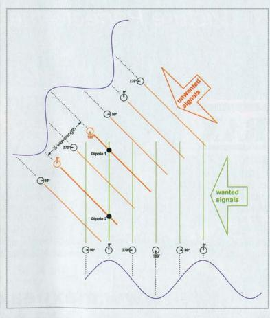
The wanted signals are received by the two dipoles exactly in phase, so the signals will be added in the combiner to give about 3dB of extra gain. The unwanted signals, however, are received exactly out of phase, so they will cancel each other out in the combiner
