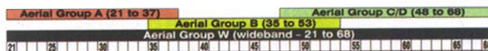
Channel groups for UHF TV aerials in the UK. The colours are the standard colour code for each group. The aerials show the relative dimensions for each group.
