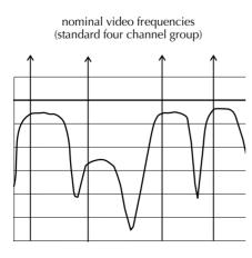
Fig. 4. Frequency response of a four channel pass filter. One channel has been set at -10dB
