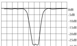
Fig. 5. Frequency response of a double notch filter, with the tuning staggered slightly. A deeper and narrower notch is obtained if the two stages are tuned to precisely the same frequency.
