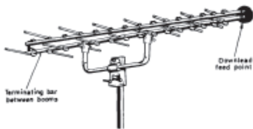
Fig. 1. The Jaybeam LBM2 log-periodic aerial
