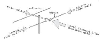
Fig. 5. Two-element aerial for VHF-FM radio. When this array is installed for horizontal polarisation there are deep, narrow nulls to each side. These can be aligned on an interfering signal in order to minimise it. This illustration greatly simplifies the polar response of the aerial, which in reality is fairly complex and irregular.
