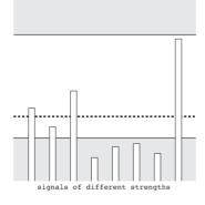
fig 2 (b). If an attenuator is used to prevent the cross-modulation, all signals will be reduced by the same amount. The signal/noise ratio of the medium-strength signals may then be inadequate for good reception. The weak signals will fall below the noise floor, which means that they will, in effect, disappear.
