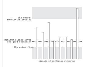
fig 2(a). Schematic, representing signals of different strengths, including one which is strong enough to cause cross-modulation.
