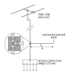
Fig. 6. The quarter-wave stub can be fitted anywhere.
