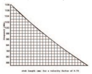
Fig. 7. CT100 cable and near equivalents have a velocity factor of approximately 0.78. this graph shows CT100 quarter-wave stub lengths for the VHF-FM broadcast band.
