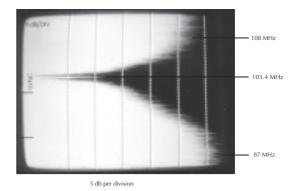
Fig.8. Spectrum analyser screenshot showing a response notch obtained with a quarter-wave stub, centred on 103.4MHz. This was set up in a workshop half a mile from a medium-powered transmitter on that frequency, and a tiny signal can be seen at the bottom of the notch. This signal has entered between the notch filter and the analyser, despite the use of good screening techniques.
