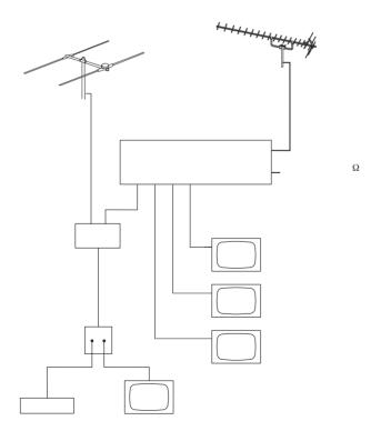
Fig 3. Where only one outlet needs VHF radio signals, the VHF aerial can be connected after the amplifier using a diplexer.
