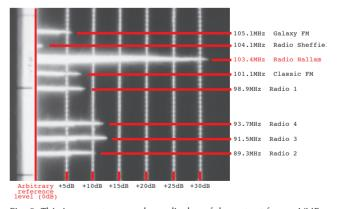
Fig. 9. This is a spectrum analyser display of the output from a VHF-FM aerial. The aerial has been aligned to minimise reception of a 103.4MHz transmitter about 1km away, but that signal is still about 20dB above the next strongest. If a 20dB attenuator was fitted to prevent cross-modulation many weak signals would be lost.
