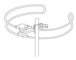
Fig. 4. The 'halo' aerial for VHF-FM radio is non-directional and horizontally polarised. The diameter is approximately 500mm.
