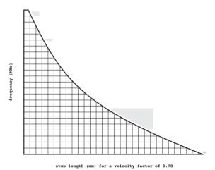
Fig. 12. Amateur radio and private mobile radio base station transmissions are amongst the many VHF signals that can enter a distribution system via the VHF-FM aerial. Quarterwave stubs or other notch filters can be used to great effect here because the width of the notch is unlikely to be a problem
