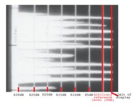
Fig. 11. Moving the reference point to the top of the display reveals a large number of weak signals. A good tuner will receive all the signals shown here, but if the distribution amplifier input is unduly attenuated to accommodate an over-strong signal, the weak ones will be lost under the noise.
